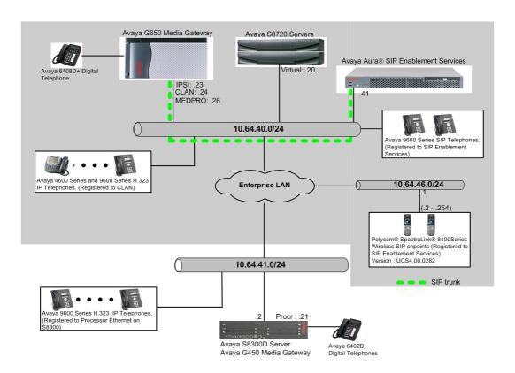
Figure 1: Test Configuration of SpectraLink 8400 Series
